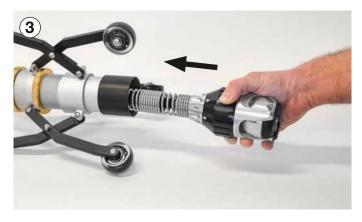
Move the camera back into the roller skid as far as it will go. The probe automatically centers itself in the guide.
