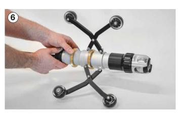
Now adjust the running gear to the required size and secure the setting with the second knurled disk.
