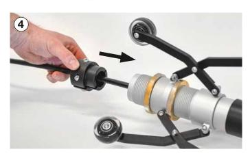
Apply the clamping lock to the push rod and slide it into the roller skid. Pull on the push rod so that the camera is tight and centered in the guide.
