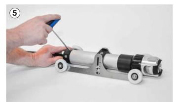
Fix the clamping lock with the two no. 5 Allen screws. This secures the camera in the roller skid.
