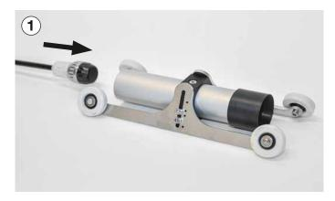
Insert the push rod through the roller skid.
