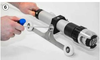
Now adjust the running gear to the required size and secure the setting with the Allen screws.
