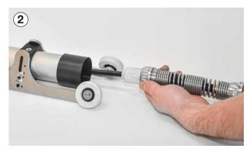
Properly connect the inspection camera to the camera connector on the push rod. (Please note: when using the CAM025 axial camera, mount the original skid beforehand).
