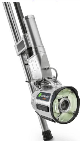
The **QuickView airHD** manhole zoom camera was developed to enable the rapid assessment of the condition of sewers. It allows sewers to be assessed from the manhole in order to plan further cleaning, inspection or rehabilitation measures. With its HD resolution and wide zoom range, sections of up to 120 m can be viewed "zoomed in". The QuickView is equipped with efficient LED haloptic lighting, a special optical system that provides ideal illumination for long distances.
