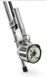
The **QuickView airHD** manhole zoom camera was developed to enable the rapid assessment of the condition of sewers. It allows sewers to be assessed from the manhole in order to plan further cleaning, inspection or rehabilitation measures. With its HD resolution and wide zoom range, sections of up to 120 m can be viewed "zoomed in". The QuickView is equipped with efficient LED haloptic lighting, a special optical system that provides ideal illumination for long distances.
