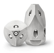
The **three-sided pick nozzles** are used for picking up hard blockages of any kind, such as mineral deposits, ice, mud crusts, sand, hardened grease, etc. The pick nozzles generate kinetic energies and ram the pick blades into the deposits. The front nozzles penetrate the material, cut it up and flush away the loose material.
