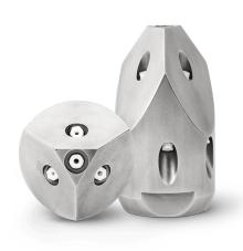
The **three-sided pick nozzles** are used for picking up hard blockages of any kind, such as mineral deposits, ice, mud crusts, sand, hardened grease, etc. The pick nozzles generate kinetic energies and ram the pick blades into the deposits. The front nozzles penetrate the material, cut it up and flush away the loose material.
