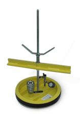
The **manhole tester** is perfect for leak tests of standard sewers with vacuum or water according to DIN EN 1610. This test is a requirement of standard DIN EN 1610 and always has to be accomplished with acceptance of construction works. The standard method fills the manhole with water and measures the sunken water height after the defined test time. However, this method is rather complicated (water consumption, prefilling time etc.), so it is often replaced with a vacuum test instead.
