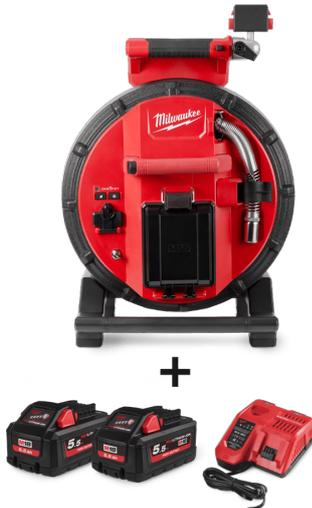
The new version of the **M18 SIC30 push camera system** now has an HDR image sensor for improved image quality and also comes with an built-in tilt sensor. Compared to the M18 SIC36, the system has a slightly thicker push cable (9.5 mm) with a length of 30 m and enables inspections in pipes from 50 - 160 mm. The thicker push cable makes it easier to push longer distances, but it is still flexible enough to pass through 50 mm 90-degree bends.
