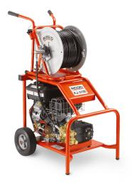
The **KJ-3100 mobile high-pressure sewer cleaner** with petrol engine is specially designed for cleaning and unblocking sewer pipes with a diameter of 50 to 250 mm. Equipped with an extremely flexible, 61 meter long hose, this high-pressure cleaner reliably removes deposits such as sludge, soap residue, dirt and grease. Thanks to the integrated pulsing system, bends and siphons/odour traps can be overcome effortlessly, allowing the hose to penetrate deeper into the pipes.
