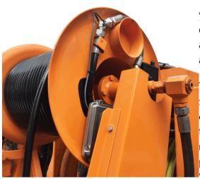
The **truck version** of the Jetcam 40 is mounted directly on your high-pressure flushing vehicle - Plug'n'Play: Slipringless, can be mounted directly on the existing reel, hose, control box and battery on it and off you go! Cleaning, inspection, bending and documentation in one operation.
