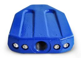
The **Flounder** is a sewer cleaning nozzle in wedge shape, the entire water output of the nozzle is directed to the sewer bottom to be cleaned. It is particularly suitable for heavy sandy or dusty deposits. The water deflection in the thrust part ensures optimum pulling properties.
