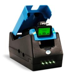
Docking station for function checks of portable gas detectors G450 / G460 / G888 / G999. With the DS400 docking stations, function tests and adjustments of portable gas detectors can be carried out fully automatically, quickly and easily. The charging function ensures that the gas detectors are ready for use when they are needed. Gas detectors that are tested every working day increase safety in the workplace. They are operated via the display and the buttons on the inserted gas detector.
