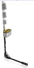
The **Digitial Manhole Measuring Device DiaMeter** is a laser measuring device for pipe diameters. It can be used to measure diameters of inlets and manholes quickly and easily. By means of an articulated joint, the measuring head can measure manholes in a vertical position and inlets in a horizontal position. The depth is determined by means of an included laser range finder.
