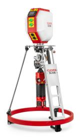
The **CleverScan manhole inspection system** was developed for one-man operation, mobile use and high productivity. Even manholes that are difficult to access can be easily detected with this system. At the push of a button, CleverScan performs a fast, fully automated manhole inspection in less than 1 minute. This means that up to approx. 50 manholes can be inspected per day by a single person.
