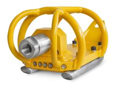
The **Bulldozer clearing nozzles** are very heavy sewer cleaning nozzles whose entire water output is concentrated on the sewer bottom to be cleaned. They are particularly suitable for heavy sandy, muddy or stony deposits. The nozzles have replaceable skids made of hardened steel.
