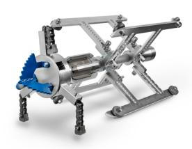
The **Blue100 Spider HD chain scrapper** "Heavy Duty" reliably removes roots and works at least as well as a milling tool. The flywheel plate with its kinetic energy is the basis for further applications such as the saw blade, the milling head or the diamond cutter.
